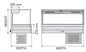
Note: For overall height dimensions, add height of motor cage (450 mm).
